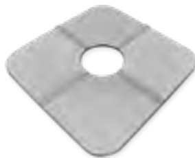
Comparators (Grit and Shot) Visual/tactile guide to surface roughness (ISO 7079). Four segments having differing degrees of etch.
