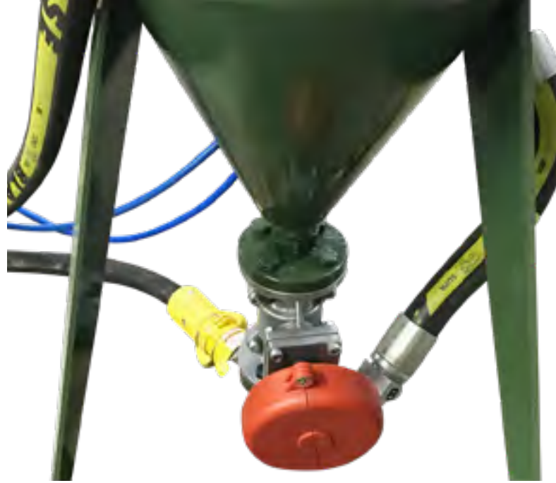
Anti-tamper guard (orange) fitted to an abrasive metering valve
