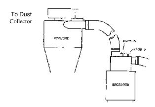
IMPORTANT NOTICE: THE INLET DAMPERS ON THE DUST COLLECTOR SHOULD BE IN THE FULLY OPEN POSITION FOR MOST COMMON ABRASIVE TYPES AND GRADES. THESE DAMPERS ENABLE MORE FINITE SEPARATION TO BE ACHIEVED WHEN FINE GRADES OF LIGHTER MATERIAL IS BEING RECYCLED.
